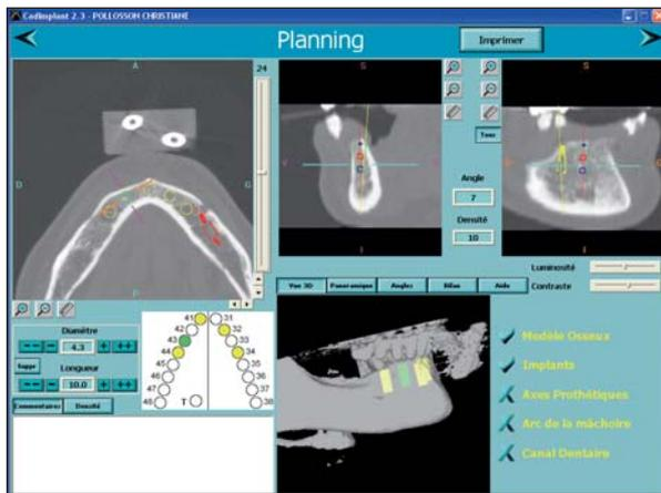
**Fig 2** CADImplant planning software was used for 3D planning. Reformatted views always passed through the planned implant axis. The practitioner could interactively change the position of the planned implant on each plane until the result was satisfactory. A simulation was carried out in real time on the 3 planes.
